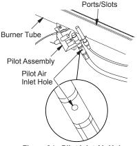
Figure 34 - Pilot Inlet Air Hole
